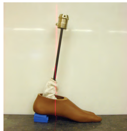
Pylon tilting forward due to excessive heel height
